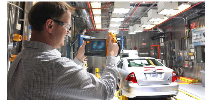
Argonne's Thermal Test Cell provides capabilities for testing vehicles under extreme temperature conditions.
