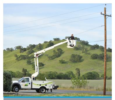
Hybrid utility truck allows for work on utility lines without engine idling. *Photo credit: Altec, Inc..*
