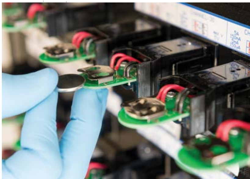
Researchers test new battery electrodes with special cell testing equipment.
