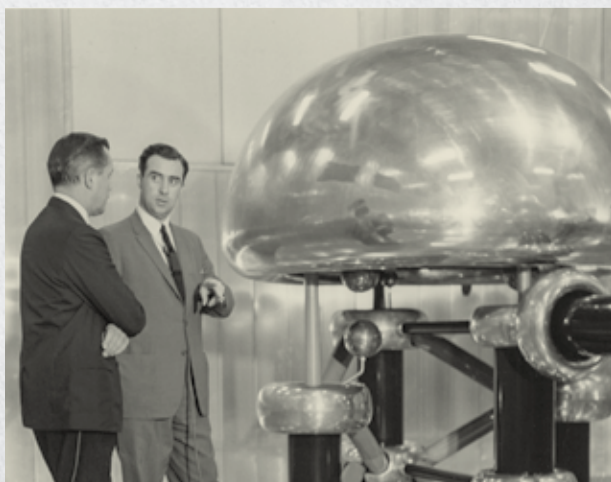
Argonne director Albert Crewe stands next to the Cockcroft-Walton preaccelerator that fed the lab's Zero Gradient Synchrotron—the nation's first high energy physics user facility. Ca. 1962.
