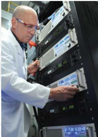
Researcher John Basco prepares for battery testing at Argonne’s Electrochemical Analysis and Diagnostics Laboratory. With the lab’s state-of-the-art, custom-built equipment, simulations are performed to provide information on battery characteristics such as life cycle and calendar life.
