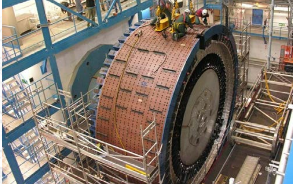
The Large Hadron Collider in Europe helps scientists explore the laws of the universe by smashing particles. Above: Argonne helped design, prototype, and build a key piece called the ATLAS Tile Calorimeter.
