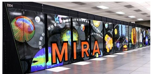
Figure 13: MIRA, a supercomputer capable of operating at 10.1 petaflops, is part of the ALCF
