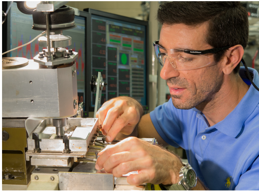
Principal Mechanical Engineer Nick Demas examines a steel specimen with a reciprocating tester.
