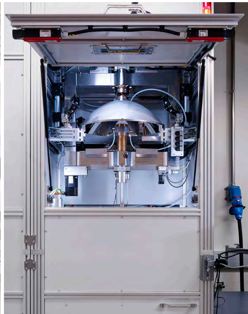
The SciDre GmbH Smart Floating Zone optical image furnace permits growth of large, impurity-free crystals at pressures ranging up to 150 bar. Control of chemical reactivity in this way leads to discovery of compounds not found under ordinary atmospheric conditions. It was brought into the lab through the oversized doors from the wide service corridor into the lab, an example of how the labs are designed to receive all sorts of equipment, no matter how large and ungainly.
