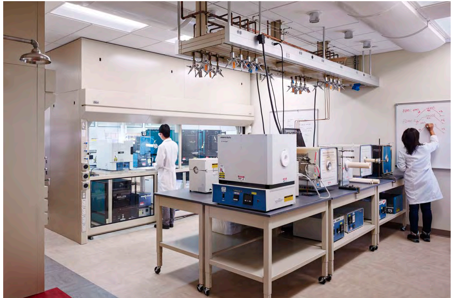
High-temperature furnaces allow precision synthesis and crystal growth of new materials under controlled atmospheres and up to 1700 degrees Centigrade. Customized furnace enclosures were designed to contain and exhaust the heat and fumes from multiple collocated furnaces and ovens.
