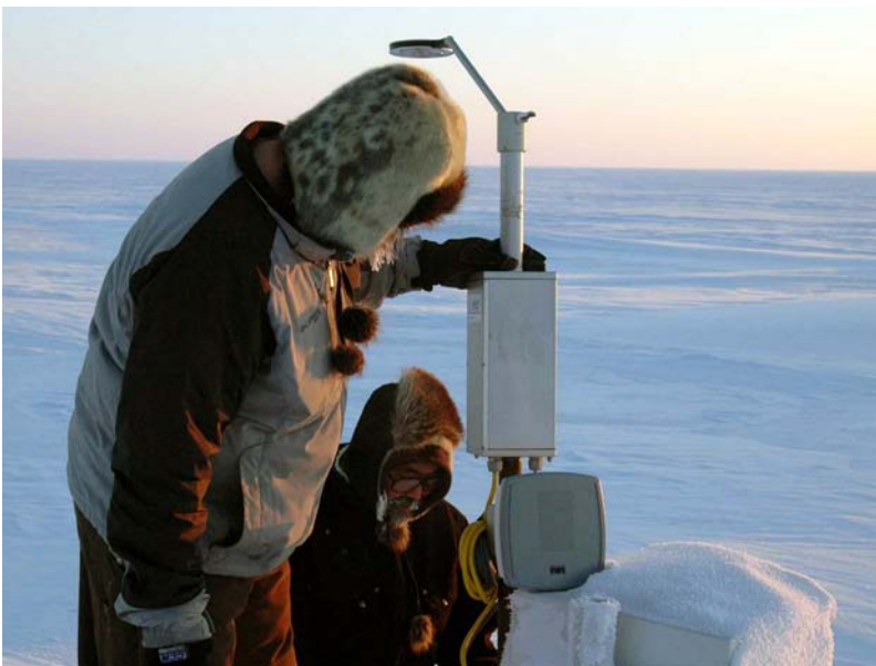
Two ARM researchers install a precipitation sensor on the tundra outside of Barrow, Alaska.
