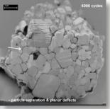
Electron microscopy images of a Li-ion battery material (NCA cathode) as prepared (left) and after 6,000 cycles of use (right) show primary particle separation and defects in highly cycled samples, which are absent in as-prepared samples. These changes reduce battery performance during continued cycling. (Photos courtesy of D. Abraham and D. Miller, Argonne National Laboratory).
