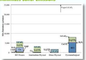
Benefits depend on the cathode chemistry; sulfur emissions reductions from using recycled material are greatest for cathodes whose elements are mined from sulfide ores.
