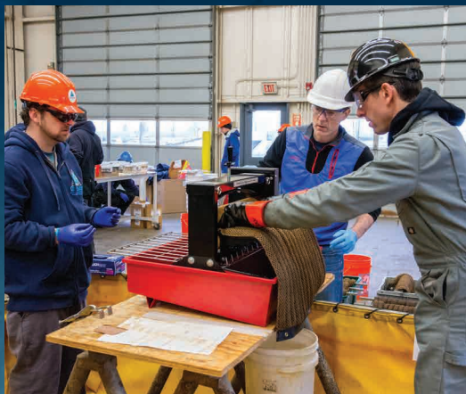
Argonne scientist Seth Darling, who co-invented the material, helps wring out the Oleo Sponge during testing. The Oleo Sponge can be wrung out, the oil collected, and the material reused — it has stood up to dozens of cycles so far without breaking down.
