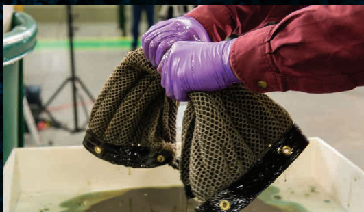
Argonne postdoctoral researcher Ed Barry wrings out a sheet of Oleo Sponge during tests at Argonne.
