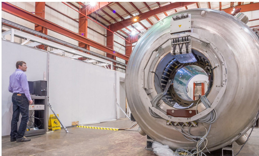
Argonne has converted this recycled hospital MRI magnet into a physics facility. This large magnet, with a strength of 4 Tesla, is used to benchmark and validate experimental equipment that will be used by Fermilab during their upcoming muon experiments, called Muon G-2 and Mu2e.
