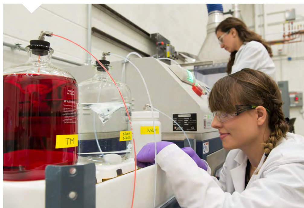
Chemical engineer Ana Kiricova (foreground) and materials engineer Ozgenur Feridun check feed solutions for a cathode precursor synthesis run on a vortex reactor.
