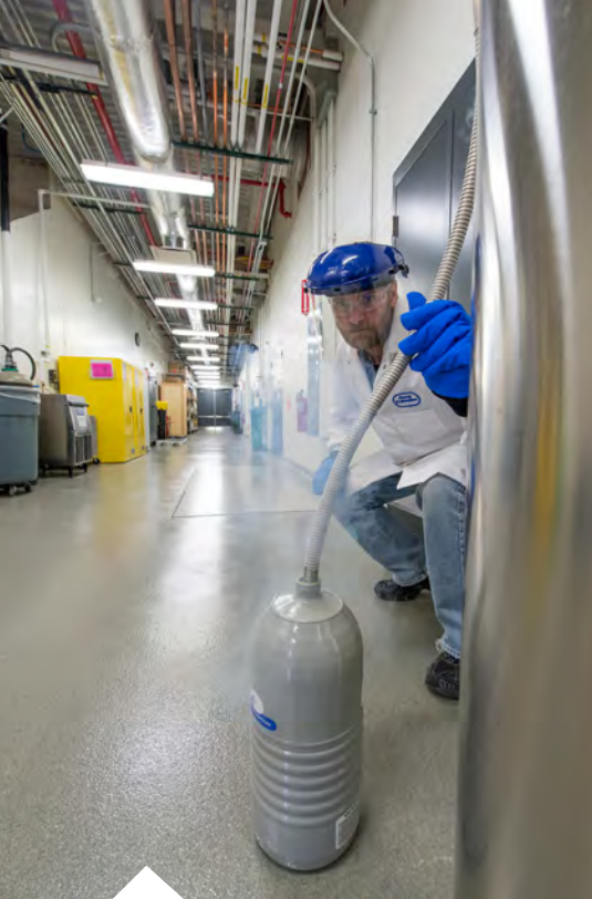
Analytical chemist Mike Kras fills a liquid nitrogen transport tank in the service corridor.
