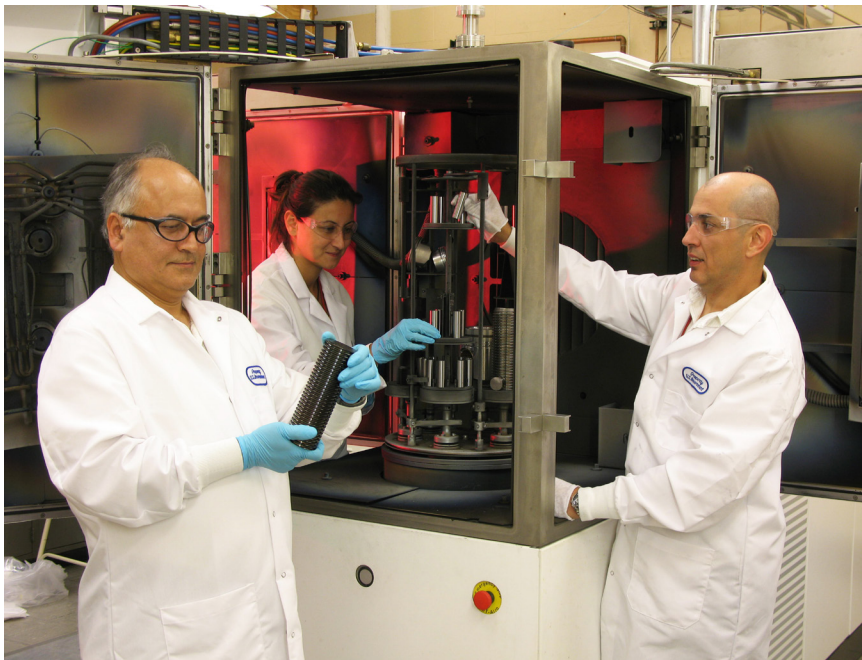
Ali Erdemir (left), student Guldem Kartal and Osman Eryilmaz load engine components into the deposition system used to coat samples with Argonne's SSC. Photo by Robert Erck.
