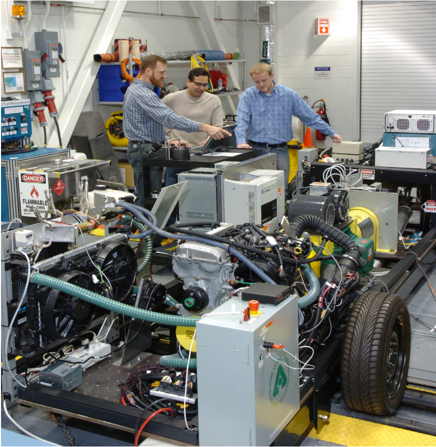
MATT – Argonne’s wheeled Mobile Advanced Technology Testbed is outfitted with scalable motor components, extensive instrumentation and a rapid prototyping control system to allow testing of plug-in hybrid electric vehicle systems.
