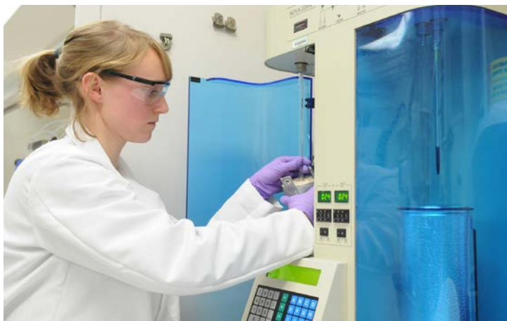
Argonne researcher Sabine Gallagher prepares a surface area analyzer for the characterization of battery materials.
