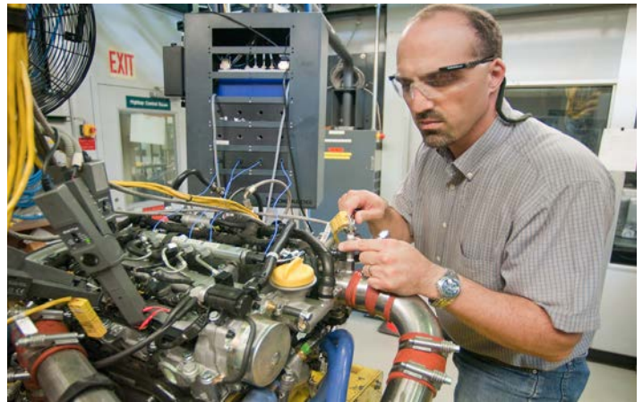
Steve Ciatti works on a diesel engine that can run on gasoline.
