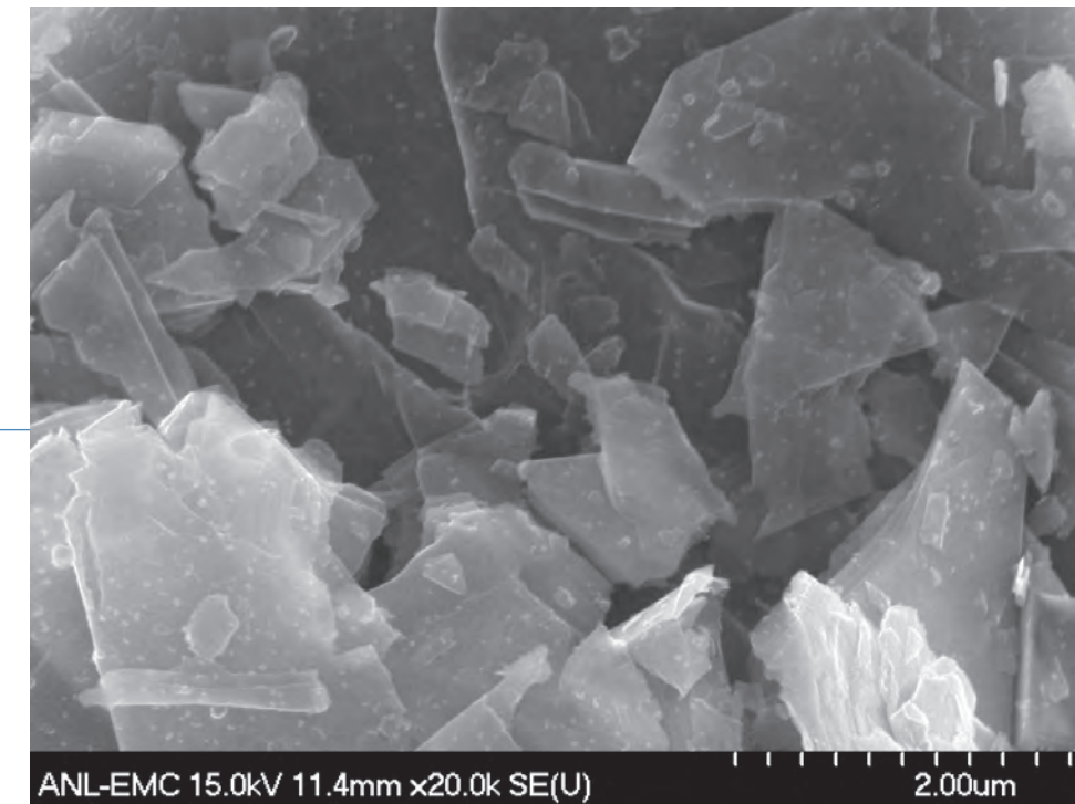
Scanning electron microscope image of \text{MoS}_2 powders, which are used in the Argonne-developed nanolubricant. Particle sizes range from 50 nanometers up to 2 microns.
