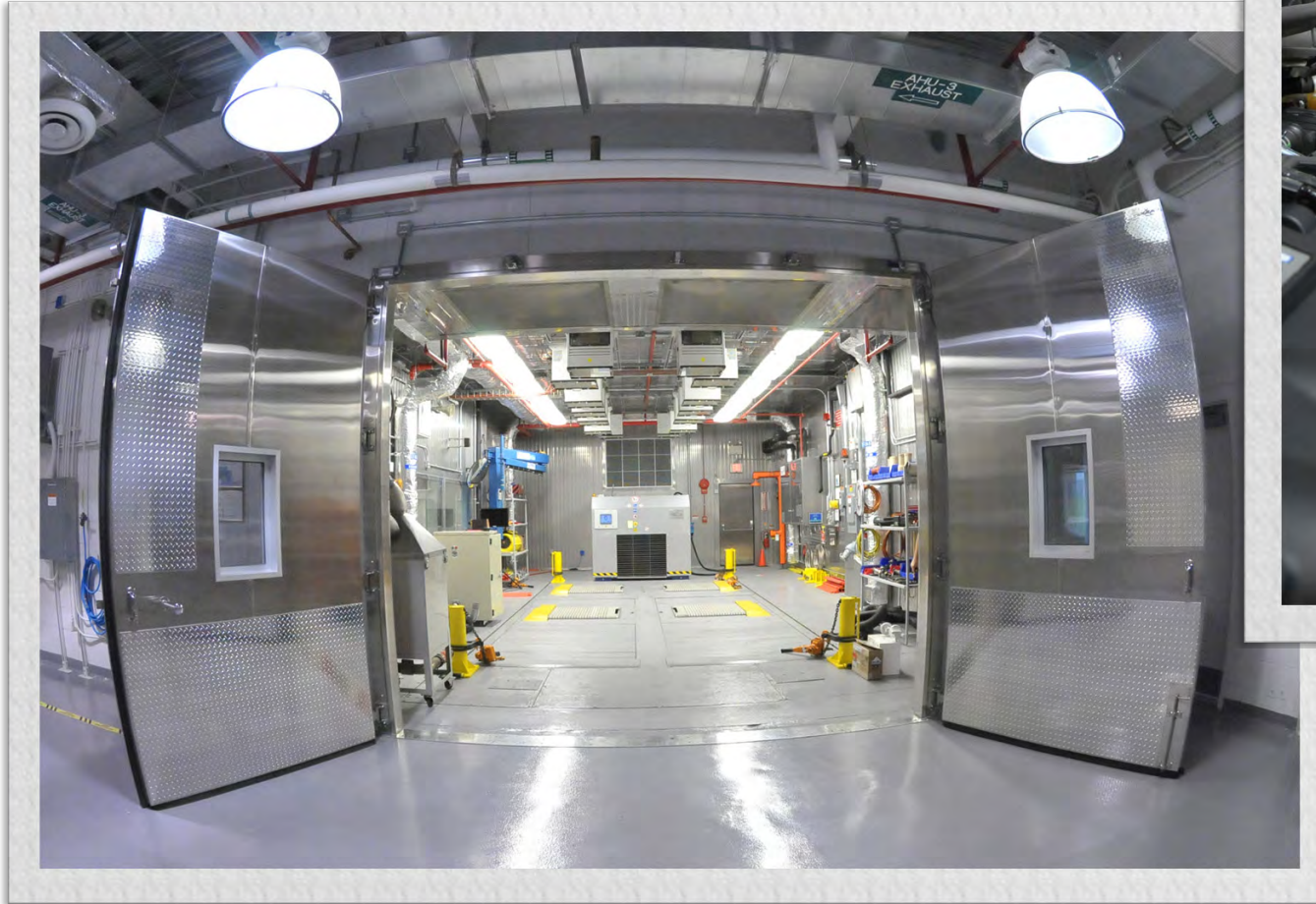
Left: Here's a first look at the Advanced Powertrain Research Facility's thermal upgrade. The new and improved facility allows researchers to test vehicles and components under extreme hot and cold temperature conditions. More on this in the next issue of TransForum.
