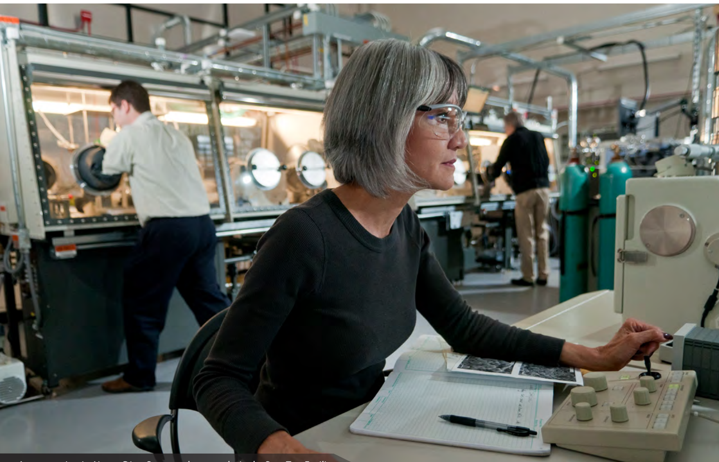
Argonne scientist Nancy Dietz Rago analyzes results in the Post-Test Facility. After a battery sample is characterized in the large glove box, it is transferred without exposure to air to the scanning electron microscope for detailed, microstructural characterization.
