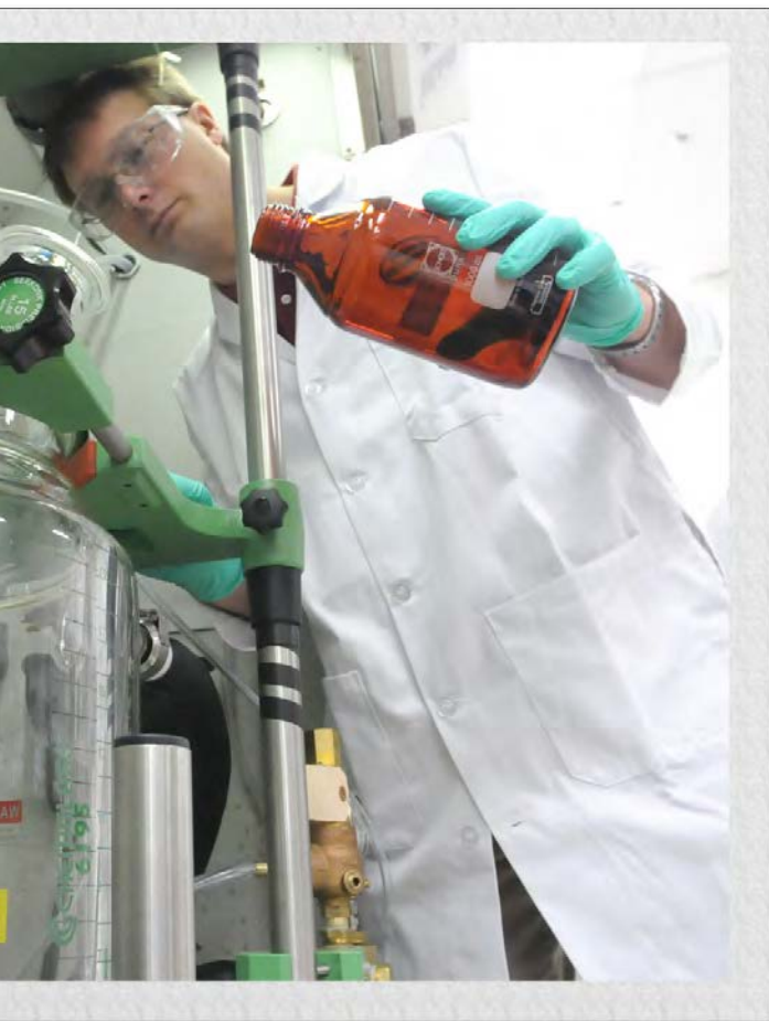
Left: Argonne process R&D chemist Trevor Dzwiniel prepares a 20-liter reactor for the synthesis of a kilo-scale batch of a lithium-ion battery overcharge protection redox shuttle.
