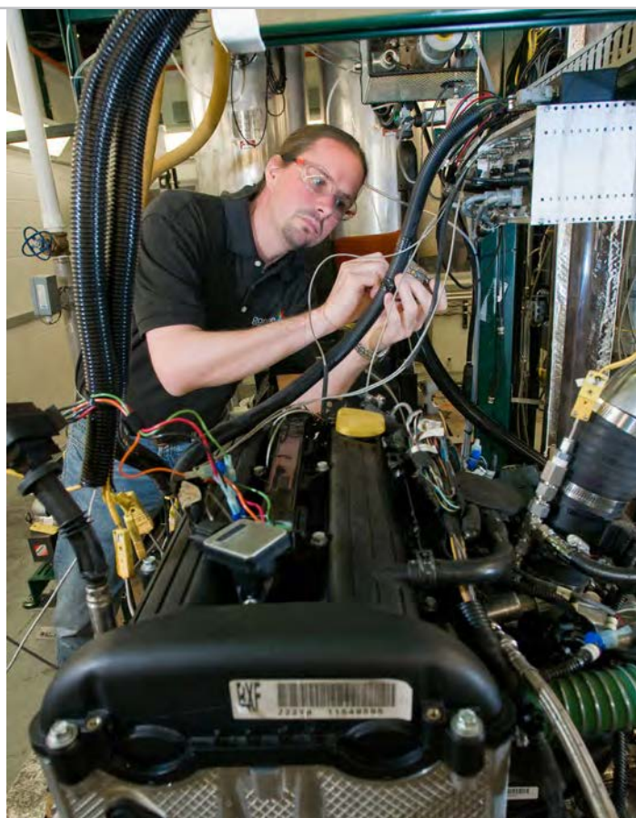
Argonne engineer Thomas Wallner adjusts the delay on an ion-sensing circuit that allows the omnivorous engine to register real-time combustion feedback.
