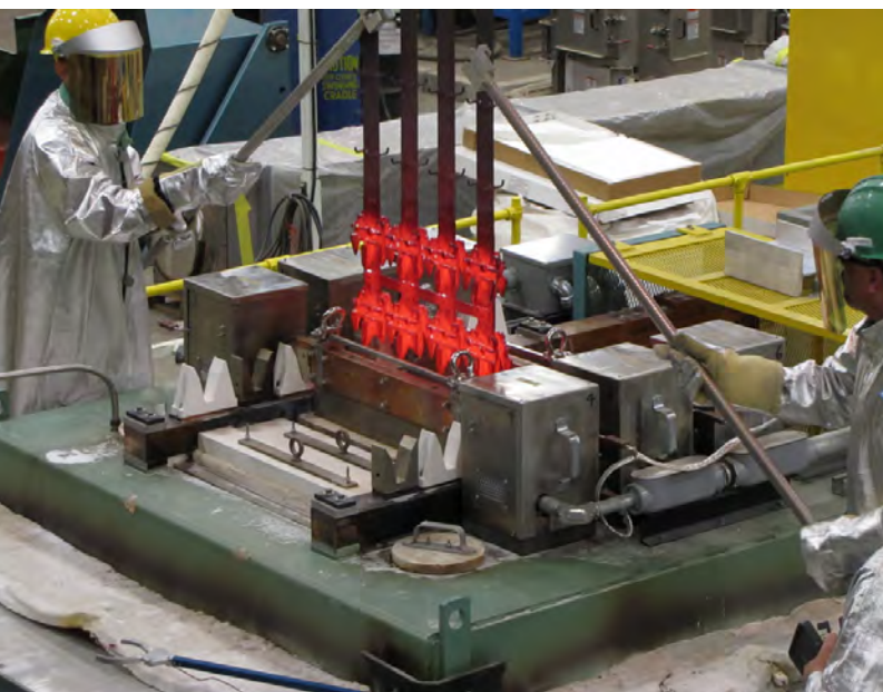
With ultra-fast boriding, metal or alloy mechanical parts are dipped into a molten borax-based solution that rapidly converts the metallic surfaces into hard, durable boride layers.
