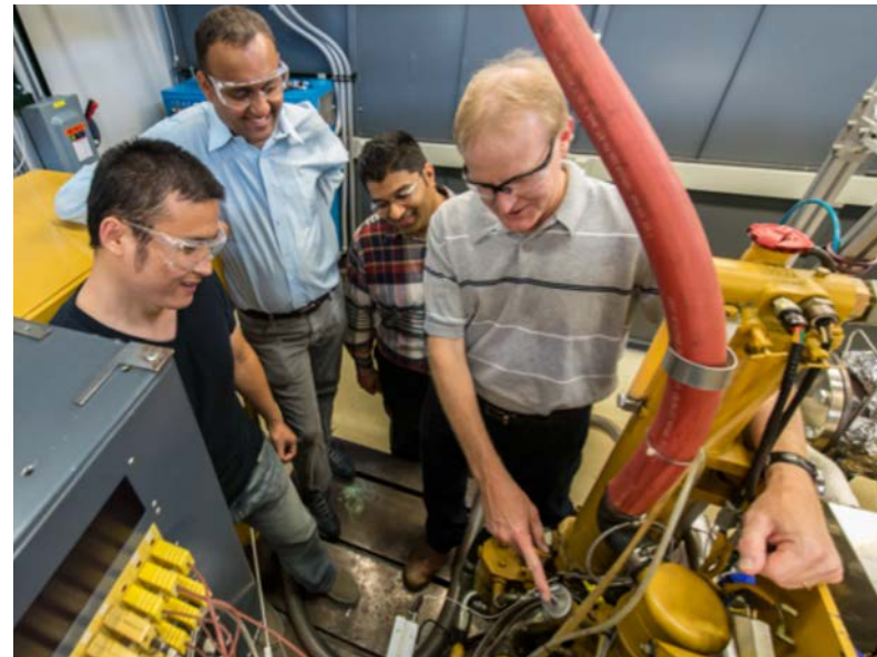
Mechanical engineer Doug Longman (right) explains to (left to right) postdoctoral appointee Yuanjiang Pei, assistant chemist Raghu Sivaramakrishnan and principal mechanical engineer Sibendu Som how the group's chemistry and modeling results will be validated using Argonne's single-cylinder Caterpillar test engine.
