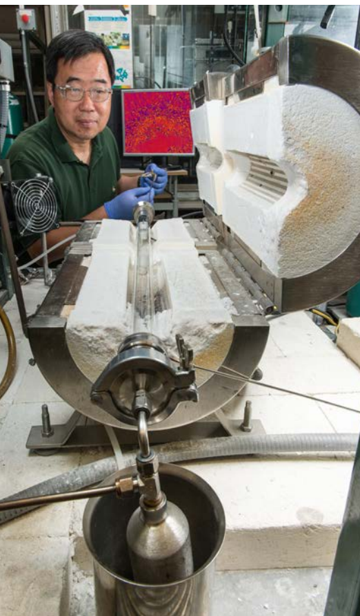
Chemist Di-Jia Liu inserts a "ceramic boat" containing an Fe/N/C composite sample into the tube furnace for thermolysis. The monitor behind Liu displays an image of electrode morphology as captured at the Advanced Photon Source.
