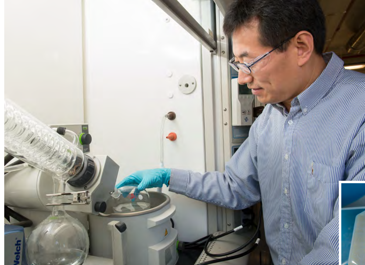
Above, John Zhang uses a Rotovap to remove solvent from the extraction solution to produce the award-winning material.
