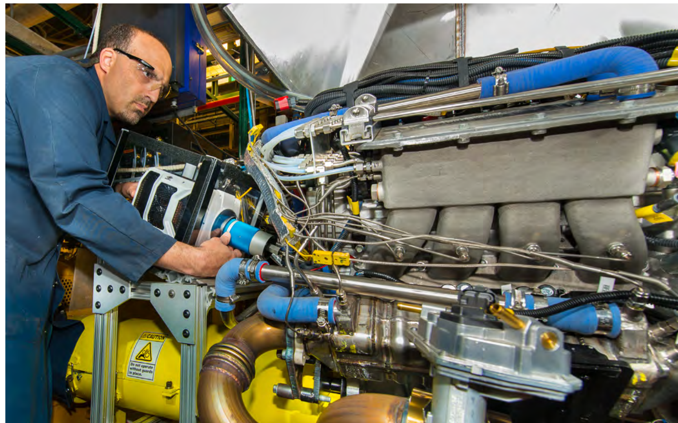
Principal investigator Steve Ciatti positions an endoscope in one of Argonne's four-cylinder LTC test engines to visualize in-cylinder combustion with high-speed (>10,000 frame/sec) movies.
