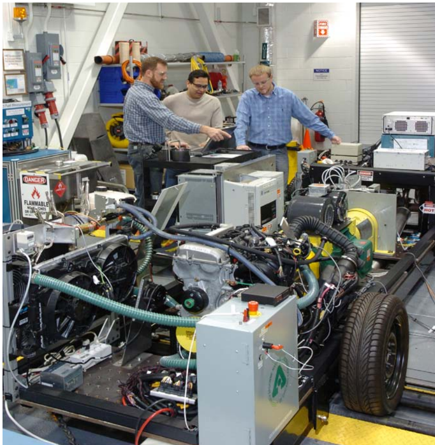
MATT – Argonne’s wheeled Mobile Advanced Technology Testbed is outfitted with scalable motor components, extensive instrumentation and a rapid prototyping control system to allow testing of plug-in hybrid electric vehicle systems.
