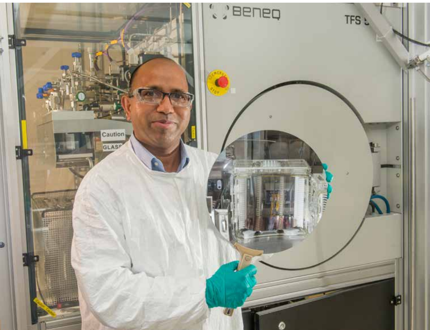
Argonne scientist Anil Mane holds a 12"-diameter silicon wafer coated with an ALD resistive film.
