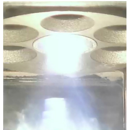
An FGC Plasma Solutions plasma-assisted air-blast injector undergoing tests at realistic conditions at NASA Glenn Research Center.
