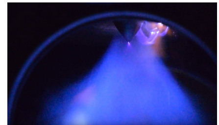
An FGC Plasma Solutions fuel injector in operation at Case Western University test bench demonstrated stabilized combustion and reduced emissions.
