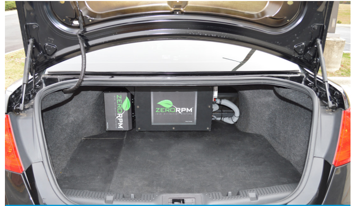
Police vehicle auxiliaries can be powered by a battery pack that fits in the trunk. Used with permission of ZeroRPM, Inc.
