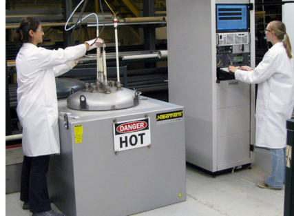
The development of an ultra-fast boriding process increased energy efficiency 80% at 15% of the cost of other coatings.
