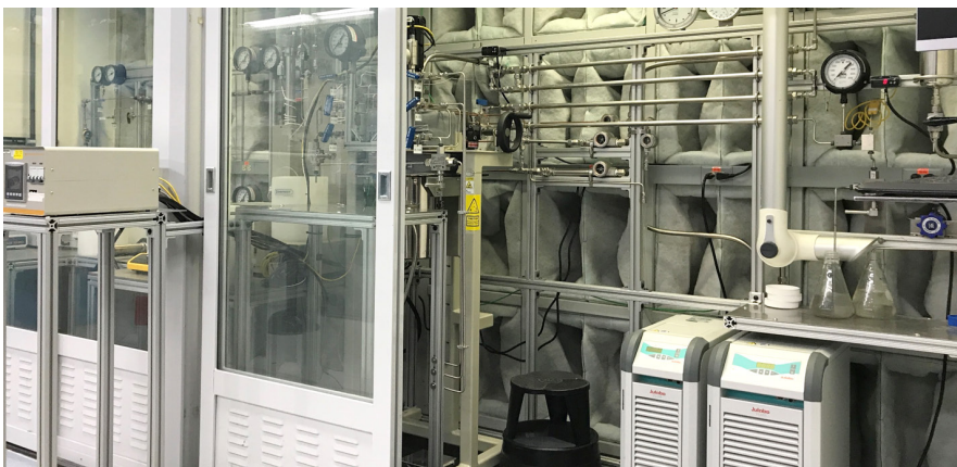
Multi-purpose Supercritical Hydro/Solvothermal Reaction Facility. The pre-pilot scale facility can produce approximately 100 grams of single crystal product per day in batch or continuous operation mode.
