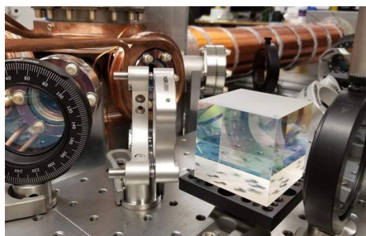
Figure 3.9-2: Optical components in the new TRACER ATTA instrument. (Image by Mark Lopez, Argonne National Laboratory.)
