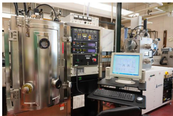
Figure 3.6-1: New evaporator and control terminal in the Target Fabrication Laboratory at CATS. (Image by Mark Lopez, Argonne National Laboratory.)
