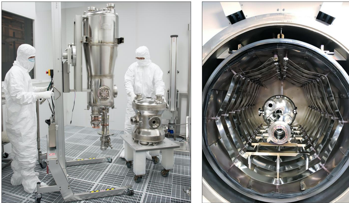
Figure 3.1-4: Argonne superconducting cavities being cleaned at the joint Argonne/FNAL Superconducting Cavity Surface Processing Facility (left) and the superconducting cavities being hydrogen degassed in a UHV vacuum furnace (right). (Images by Argonne National Laboratory.)
