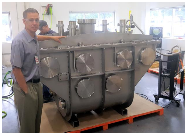
Figure 3.1-3: Bunch Lengthening System cryomodule for the Advanced Photon Source Upgrade. (Image by Argonne National Laboratory.)
