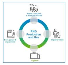
RNG can be produced and used in a closedloop process. Biogas systems use anaerobic digestion to recycle organic waste, turning it into energy and liquid and solid coproducts valuable in agriculture.
