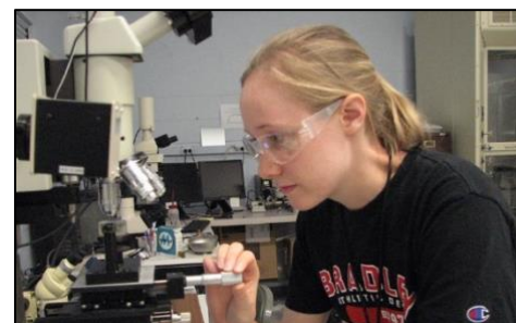
Alyssa Skulborstad (2009 Undergraduate Summer Intern) conducts measurements of a new coating developed at Argonne National Laboratory using a “microhardness” test machine. This new coating process produces a valuable, hard, wear-resistant layer on steel materials. (Source: Argonne)
