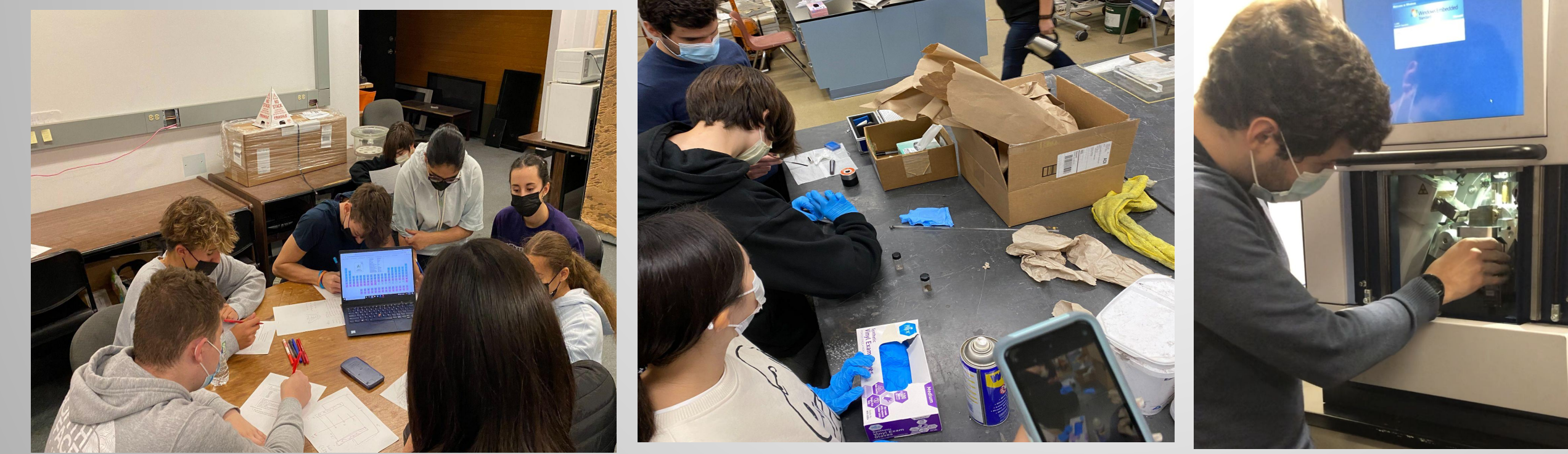
Figure 2. Left image depicts students performing stoichiometry calculations to determine the amount of each compound needed for formation of the desired HEO electrode. Center image shows students making a pellet of the desired compound prior to the annealing process. The right picture illustrates the x-ray diffraction analysis used to determine whether or not the desired structure was created through the ball milling and annealing process.
