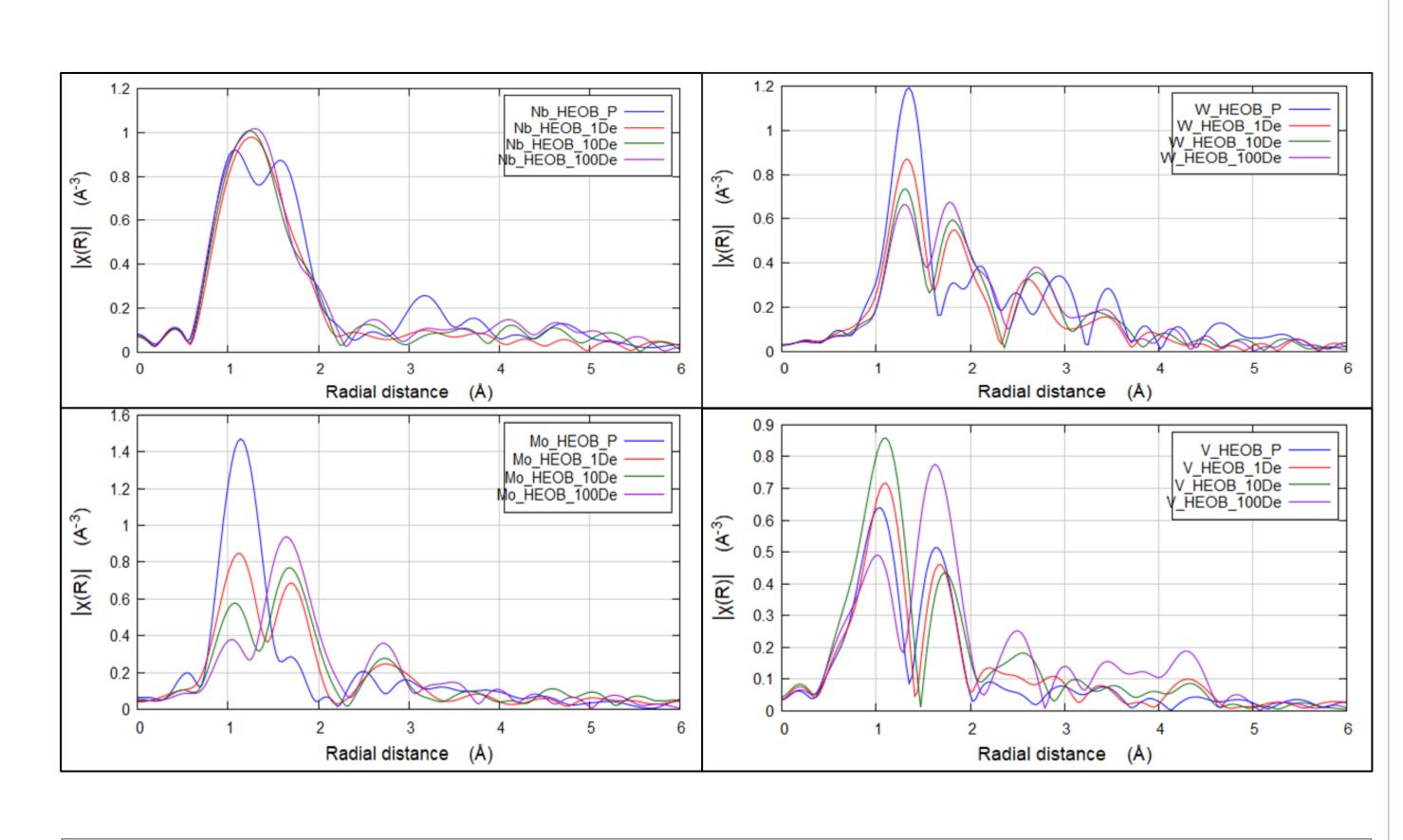
Battery cycling data shows the different delitiation states and the magnitude of oxidation over radial distance.
