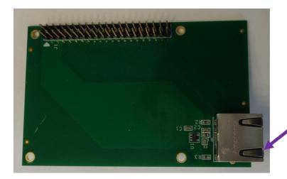
The **dongle** mounts to the **array frame** and never moves, providing a non-volatile memory of information specific to the unique array position.
