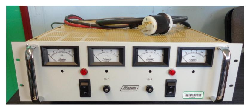
Bolted to rack with insulated mount, ground provided via cord.
