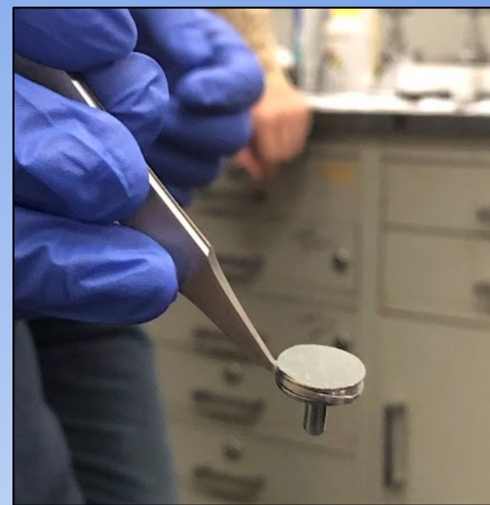
Figure 4. Cathode material formed from \text{LiVOPO}_4 , the 'test material' in this battery.
