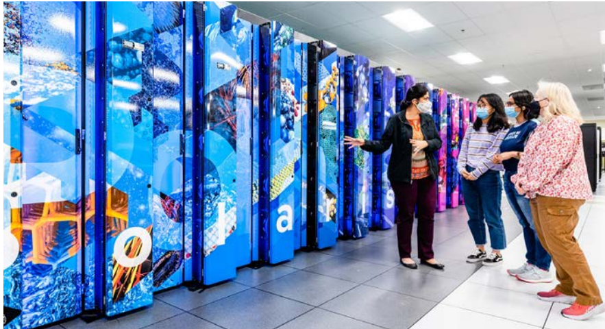
The Polaris testbed supercomputer provides researchers and developers with a powerful new platform to prepare for science in the era of exascale computing.
